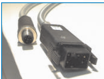
Modular design and plug-in electrical contacts facilitate quick module replacement.
