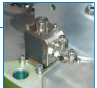
Drum blow-off valve
