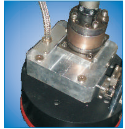
Manifold designed for single or dual hose output
