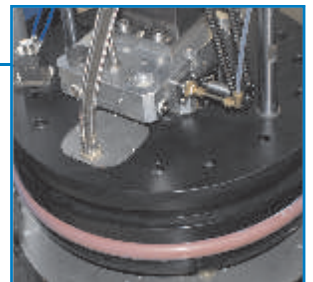
Teflon-coated platen with cast-in heaters
